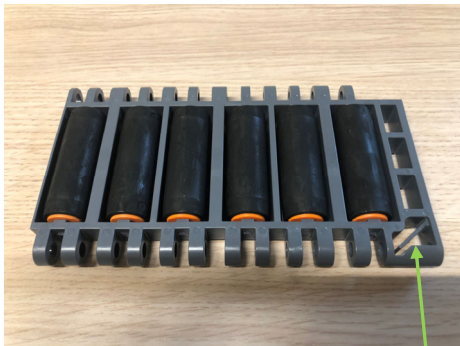
Edge module within the right corner the "barndoor" this is used to retain the rods.
